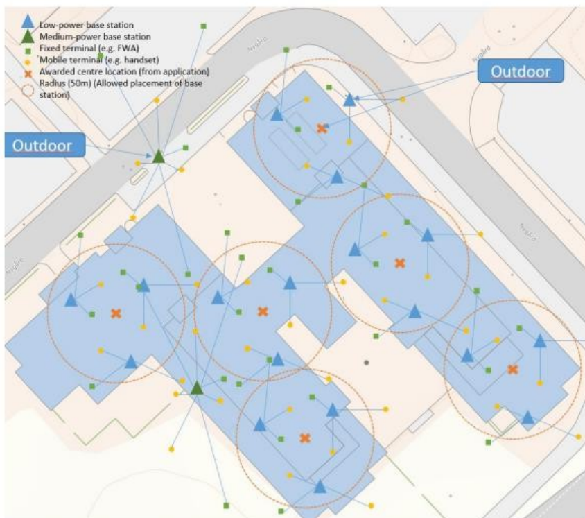
Figure 7: Multiple low-power licence areas combined, and how the uppermost licence area is deemed outdoors (if one or more low-power base stations are outdoors, the entire licence area is deemed outdoors)
